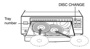
**To load three to five discs**, press the DISC CHANGE button to rotate the trays after placing two discs. Place the next disc on the empty tray. Each time the DISC CHANGE button is pressed, the trays rotate and one disc can be placed.
