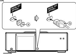
This unit can output CD digital sound signals through this jack. Use an optical cable to connect digital audio equipment (digital amplifier, DAT deck, MD recorder, etc.).
